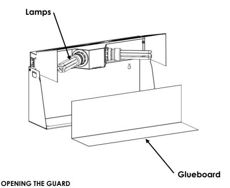
The guard can be opened for easy cleaning and servicing. To open
